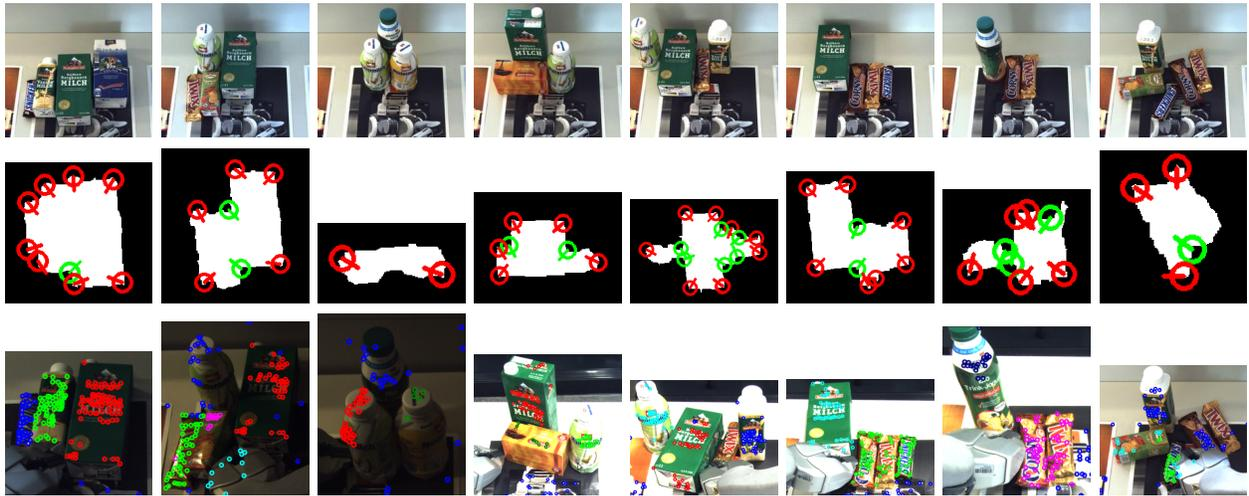
Fig. 5. Test scenes 1 to 8 from left to right. Top row: original scenes, middle row: contact point estimation, bottom row: segmentation after the first push cycle. Please note, that successfully segmented objects were removed from the scene and the contact point estimation and segmentation cycle were repeatedly executed.
