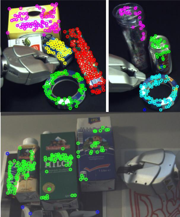
Fig. 7. Failure cases exemplified. In the left-top scene the “black pepper” object became occluded by the robot arm. In the right-top scene the features on the semi-transparent object were tracked unsuccessfully. Bottom row: failed segmentation from the random pushing experiment where the robot pushed objects such that they all moved rigidly with respect to each other
