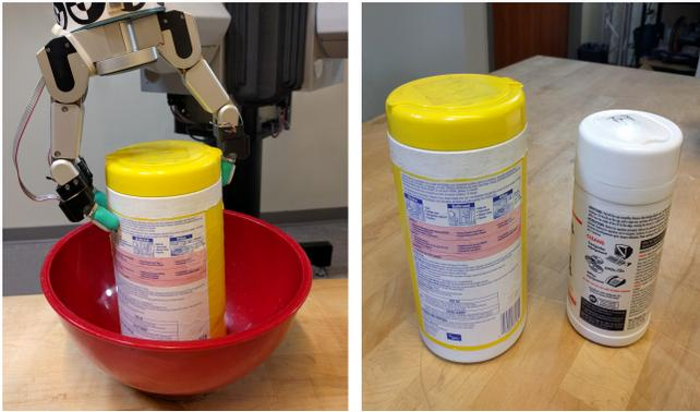
Fig. 3: *Left*: Experimental setup used for learning the grasp stability predictor and the regrasping behavior. If the object falls out of the hand, it returns to its initial position due to the convex shape of the bowl. *Right*: The novel object (on the right) used for testing the regrasping behavior in comparison to the original object (on the left).
