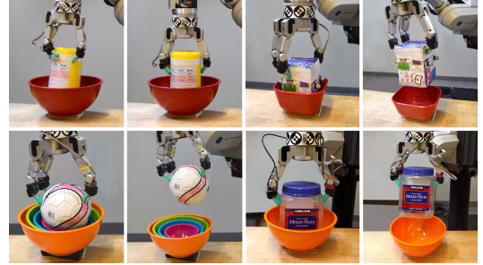
Fig. 1: Objects and experimental setup used for learning the grasp stability predictor and the regrasping behavior. Top-left : the cylinder. Top-right : the box. Bottom-left : the ball. Bottom-right : the novel object.
