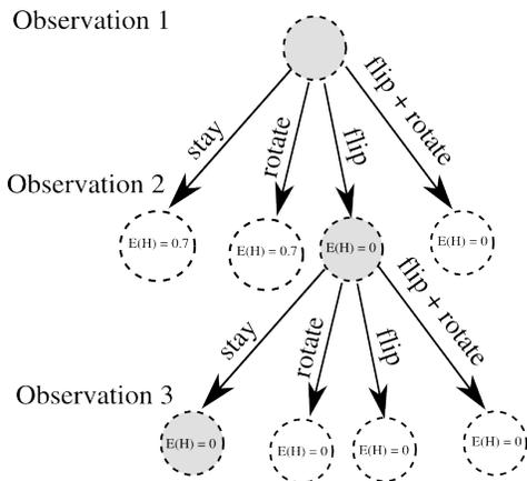
Fig. 5. Decision tree based on the action selection algorithm. Each node in the tree represents the expected entropy of the posterior probability for a given action. Colored nodes indicate the choice of the action that results in the minimum expected entropy.
