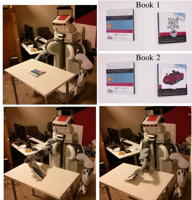
Fig. 1. Top-left: The service robot PR2 trying to recognize a book based on its back. The database of objects consists of book 1 (top-right, NE and NW) and book 2, (top-right, SE and SW) that look the same from the back. PR2 takes the optimal action in order to recognize which book it is. In this case it means it flips it over (bottom-left, bottom-right).
