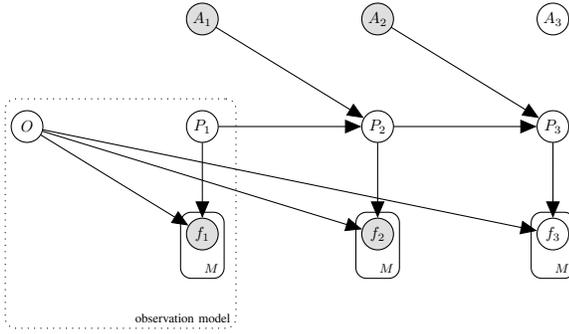
Fig. 2. Probabilistic graphical model for interactive object recognition.
