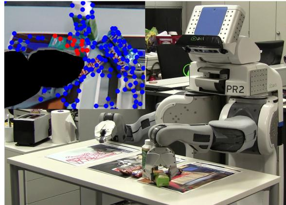
Fig. 1. Top: PR2 robot successfully picking-up the object after segmenting in it in clutter using herein proposed object segmentation algorithm.
