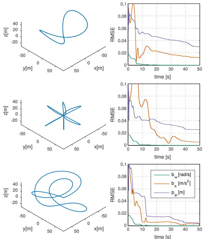
Fig. 1. Root Mean Squared Error (RMSE) convergence of EKF self-calibration (accelerometer and gyroscope biases  $b_a$ ,  $b_\omega$  and position of the GPS sensor  $p_{ip}$ ) state estimates for a) figure-eight trajectory, b) star trajectory, c) optimal trajectory from our method. We introduced additional yaw motion for a) and b) trajectories in order to improve state estimation of these heuristics.
