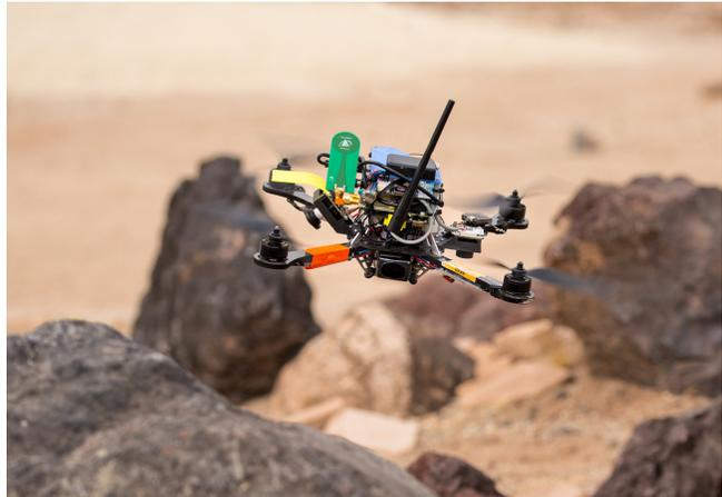
Fig. 1. The Asctec Hummingbird UAV used during the experiments.
