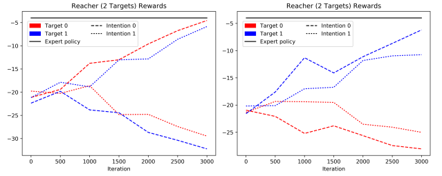
Fig. 1. Rewards of different Reacher policies for 2 targets for different intention values over the training iterations with (1) and without (2) the latent intention cost.
