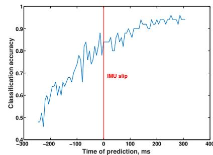
Fig. 4: Linear / rotational slip classification accuracy.
