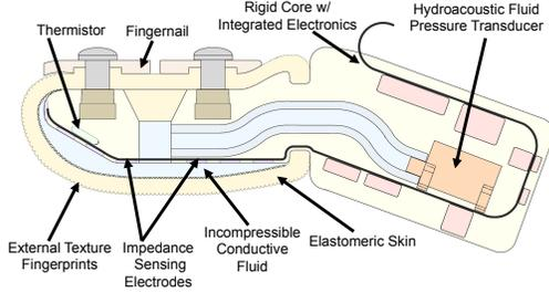
Fig. 1: Cross-sectional schematic of the BioTac sensor.
