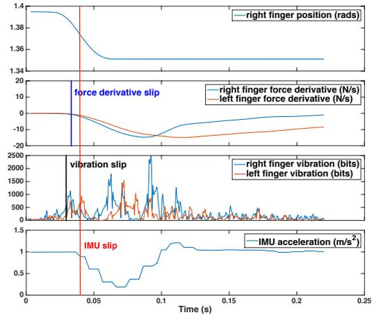
Fig. 3: An example run of the slip detection experiment.
